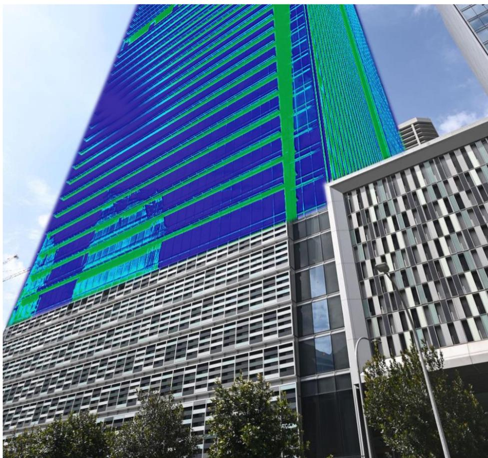
*Figure 1: Operva AI utilises drone technology, infrared thermography and AI to detect air and water leakage in buildings. (For illustration purposes only. This does not represent the actual thermal profile of the building.)*
